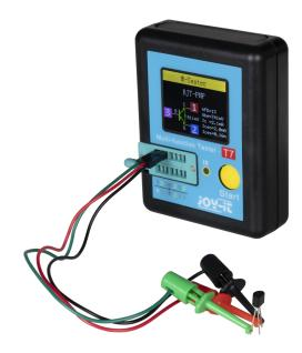
This LCR meter offers a wide range of functions at a low price. The LCR meter can measure capacitance, resistance, and inductance among other things. In addition, it can automatically recognize components, for example, it can distinguish between different types of transistors, such as NPN or PNP The transistors. device is particularly easy to operate, as all measurements are started at the touch of a single button.
