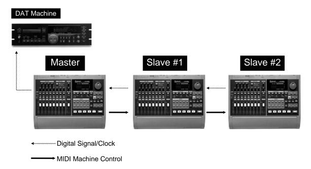
In this setup, MIDI Machine Control allows you to control the transport functions of the slave units from the master unit. Digital Clock is used to sync the timing of the three units and the Digital signal is routed through the master VS-880 so that the audio from all three units can be mixed to DAT.
