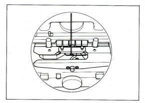
e. Continue to hold the end of yarn with left hand, and move the connected carriage from right to left.
