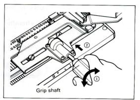
(4) Holding the ribber with both hands so that the gate pegs of the ribber are up and the purl needle butts are toward you.
