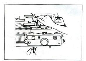
d. Pass the yarn into the yarn feeder securely.
