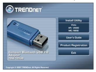
Click "Install Software (Utility)" on the menu to install the Bluetooth USB Adapter driver and software. Select "Vista", and the install wizard will begin the software installation. Follow the install wizard instructions to complete the installation.
