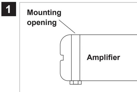
The mounting openings for the installation are located on each corner of the amplifier. Please ensure during the installation, that you don't scratch or damage the amplifier surface with the tools.
