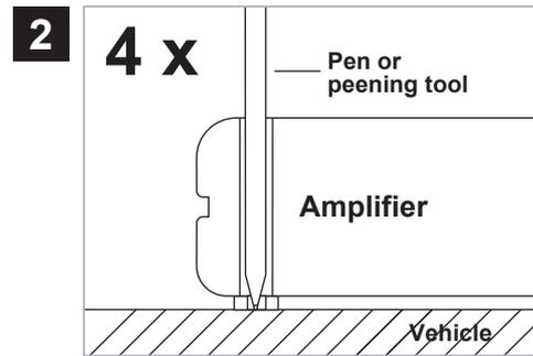
Uphold the amplifier to the chosen mounting location in the vehicle. Then mark the four drill holes with a appropriate pen or peening tool and lead through the mounting openings.
