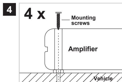
Then uphold the amplifier to the chosen position and fix the screws through the holes of the mounting brackets into the drilled screwholes.
