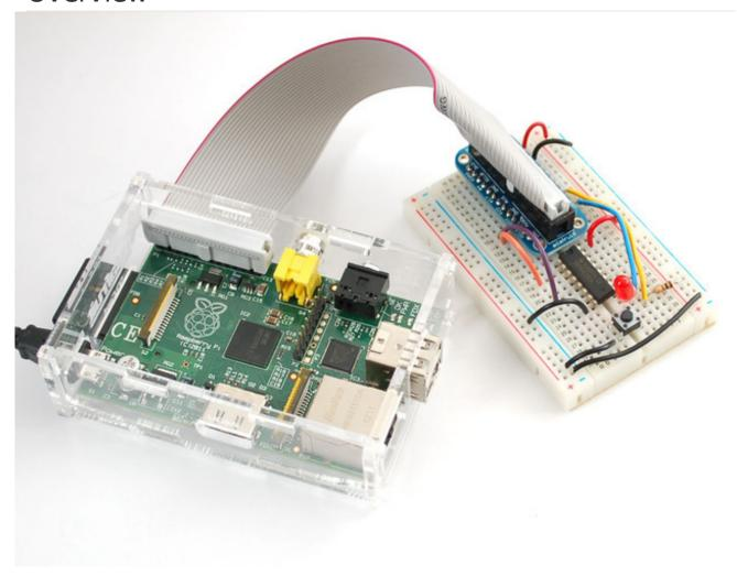
Now that you've finally got your hands on a Raspberry Pi® (http://adafru.it/aHx), you're probably itching to make some fun embedded computer projects with it. What you need is an add on prototyping Pi Cobbler from Adafruit, which can break out all those tasty power, GPIO, I2C and SPI pins from the 26 pin header onto a solderless breadboard. This mini kit will make "cobbling together" prototypes with the Pi super easy.
