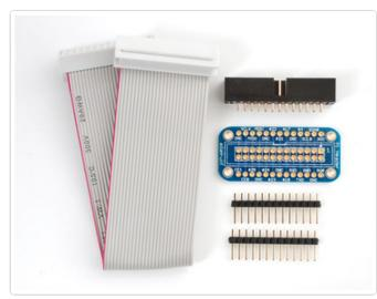
First up, open up your kit and verify you have the components - gray cable, blue PCB, black connector and a stick of male header. The header is breakaway, so it might be one long piece instead of two shorter
