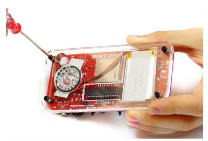
If everything electronics-related is working fine, the last step is to put the guts (electronics) in a nice crystal clear acrylic casing so that everyone can see your perfect soldering joints!
