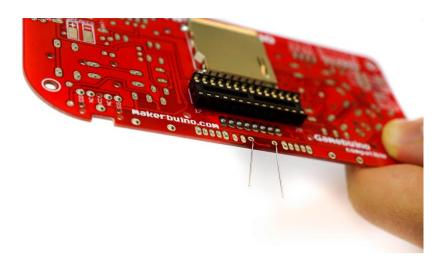
**Important:** Remember to cut all the leads of the components you've soldered using your diagonal cutter pliers.
