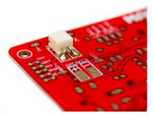
This connector is pre-soldered to MAKERbuino's PCB and is used for connecting the Li-Po battery to the circuit.
