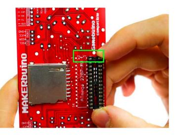
**pro tip:** first solder the two diagonal pins of the socket, then make sure that the socket is aligned with the board nicely, correct the alignment if needed and solder the rest of the pins.
