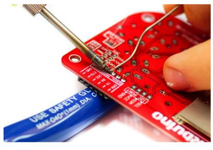
**Pro tip:** If the component is falling out of the PCB when you try to solder it, place your cutting pliers' handle underneath the component you're soldering.
