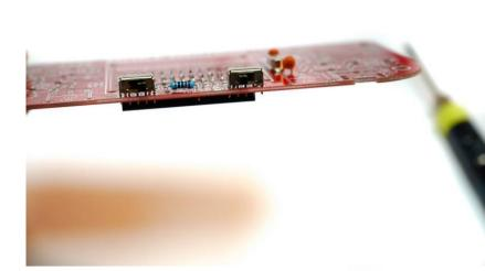
The left switch is muting the sound and the right one will turn the console's power ON & OFF. The switches have to go all the way down and sit nicely on the PCB.
