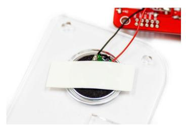
Let's fixate the speaker to the back side of the casing. We recommend using a piece of insulating tape for this. Alternatively, you can use a hot glue gun or some super glue.
