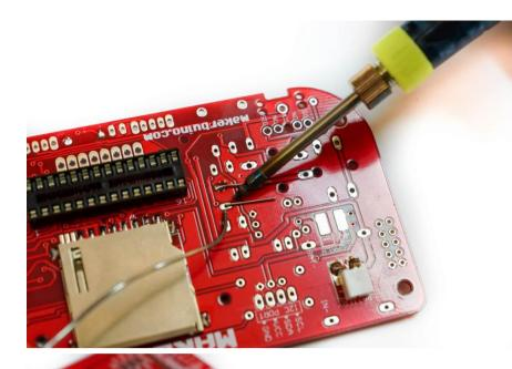
Apply the previous pro tip and bend the leads of the crystal at the back of the board.
