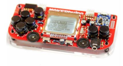
Next up, place the colored button caps to the yellow pushbuttons by simply snapping them on (you will have to apply some force and that is completely normal).
