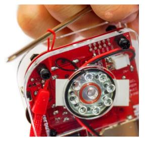
Continue by mounting the front plate and fixating it with black hexagonal M3 spacers and nuts.
