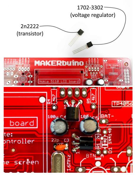
Solder the regulator on the board where "IC2 3.3V" is marked and the transistor to the spot with "T1 2N2222" marking on it. Be careful to turn these components on the right side!
