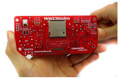
Continue by soldering the four pads of the socket's shielding.
