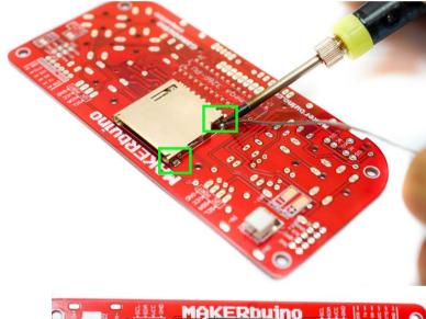
When soldering the socket's contacts, you DON'T have to solder the three rightmost pins because they are not used.
