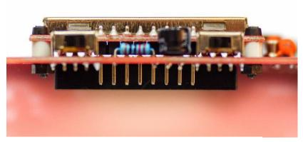
**Important:** before soldering the screen to the PCB, fasten its bottom two holes with screws, nuts, and spacers. In this way, you'll ensure that the screen module is aligned perfectly before soldering it to the PCB.
