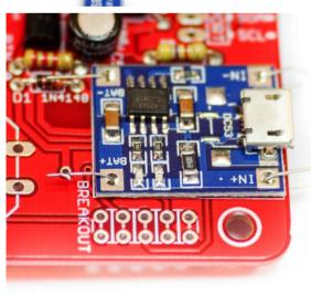
through charger's and PCB's contacts and bend them before soldering.
