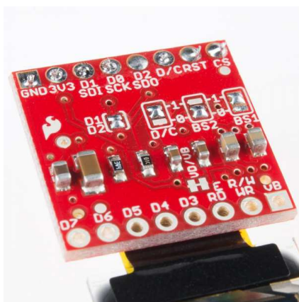
Breakout jumpers set for I 2 C mode.
