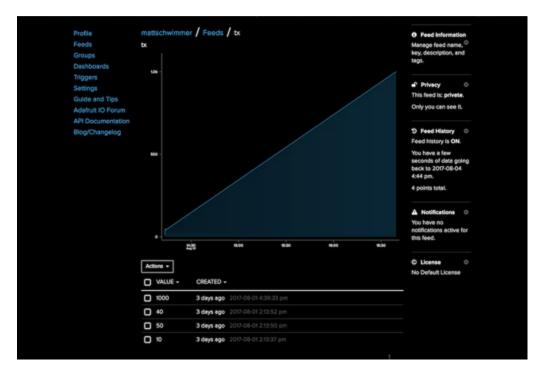
This is an example of a TX feed that presents data sent from the Bluefruit LE Connect app to adafruit.io via MQTT.
