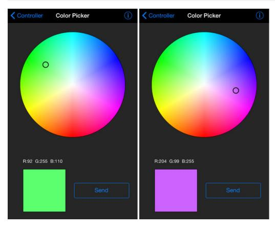
The Color Picker sends a color's RGB values to Bluefruit LE. This can be used to control the state of RGB LEDs such as Neopixels.
