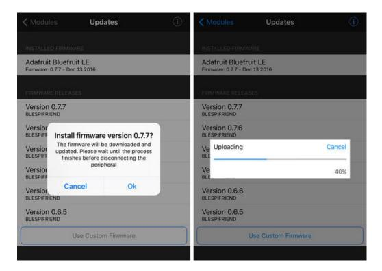
You'll then be asked to confirm the update process. After tapping **Ok**, the process will begin. Once the update process is completed, the app will automatically disconnect from the device and the device will reboot.
