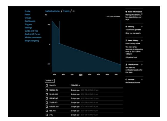
This is an example of an RX feed that presents data **sent** from an Adafruit Feather Bluefruit and is **received** by iPhone using the Bluefruit LE Connect app via MQTT. The data is sent using an ASCII Numeric format similar to how plotter data is sent. You can see the plotter feature here.
