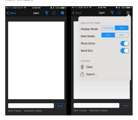
The main log window is in the middle, and will display data both received and, if Echo is on, sent.
