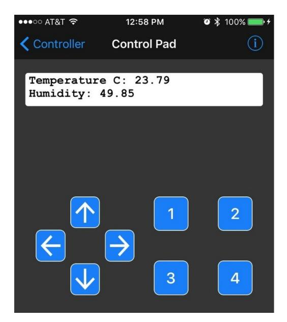
The Control Pad function provides a familiar momentary button interface for common control scenarios. Data is sent on the press and release of each button. Each packet consists of 4 bytes, each representing a char value. The first two chars identify the packet as a button message, the third specifies a button, and the fourth signifies either a press or release.
