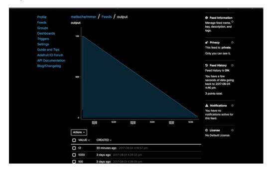
This is an example of an output feed that presents data created on adafruit.io **sent** to the Bluefruit LE Connect app via MQTT
