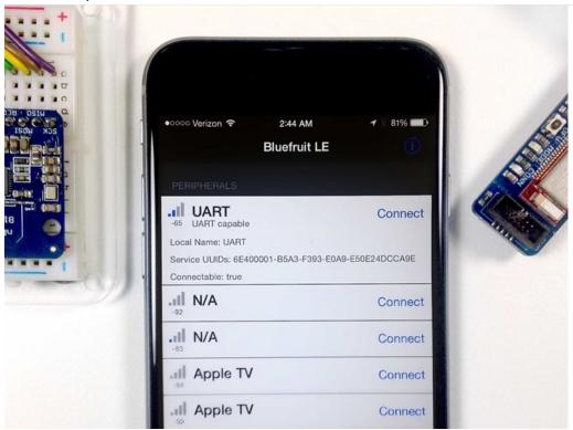
The Bluefruit LE Connect app provides iOS devices with a variety of tools to communicate with Bluefruit LE devices. These tools cover basic communication and info reporting as well as more project specific uses such as Arduino Pin Control and a Color Picker.
