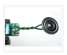
Twist the wires, this will reduce the strain on the solder joints when bending. Put the end of each wire into the two PCB holea marked SPK+ and SPK-. Don't solder into the hole in the middle which is for the battery. The speaker is 'symmetric' so it doesnt matter which wire goes in which hole.
