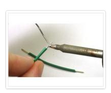
Next, it is a good idea to tin the ends of the wires. Its a little tricky because it requires holding three things. However, if you have a 'third hand tool' or a vise, you can use that to hold the wire while you heat up the stripped end and coat it with a little bit of solder. This will make it easier to connect to the speaker.
