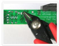
Flip over the PCB and solder it in. Then clip the leads.
