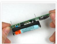
Slide the battery holder into the PCB (**but do not solder it in**). Make sure that the battery is aligned correctly. Putting in the battery backwards shouldn't damage the circuit but it's still not a good idea so try to get it right the first time. The back of the PCB has a silkscreen to help determine which way the battery goes in.
