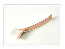
Next cut a 1.5" piece of copper tape using the diagonal cutters. Don't use scissors as the metal tape can damage them. Peel off the paper backing. The copper tape is conductive, sticky and flexible which makes it perfect for wrapping the pencil.
