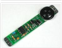
Now use the tip of your iron to quickly remelt the blobs so that they flow onto the speaker tabs.
