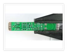
Get ready by placing the PCB in a vise.
