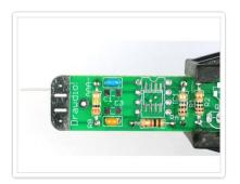
Next are the two ceramic capacitors **C1** and **C3**. Ceramic capacitors also have a nice property that they are symmetric/non-polarized. That means they can go in 'either way'. The capacitors are different values so make sure to not mix them up.
