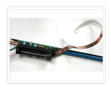
Next take 3 or 4" of copper tape and start wrapping around the bottom of the pencil, starting with the silver tab on the PCB and ending an inch before the end of the pencil. This will make contact with your hand and provide the second half of the sensor.
