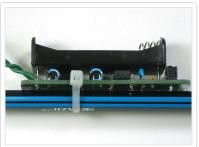
Next you can mount the PCB to your pencil. Place the PCB on the flat side of a pencil, and thread the zip tie through as shown and tighten it. You'll want it about an inch or less from the top of the pencil. The higher it is the more pencil you'll have to sharpen but it may be a little more unbalanced.
