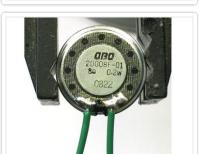
Next, warm up the tabs and slide the tinned ends of wire into the melted solder pool. Then remove the iron and wait a few seconds, the solder pool will cool with the wire in place. Do the same for the other pad.
