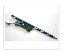
Finally, insert a battery into the kit. Then grip the pencil with one hand and touch the point of the pencil to your other hand. You will be able to hear the drawdio make noise!
