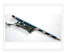
Finally, insert a battery into the kit. Then grip the pencil with one hand and touch the point of the pencil to your other hand. You will be able to hear the drawdio make noise!
