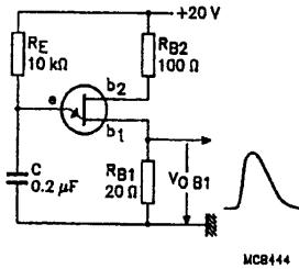
Fig.4 Impulse output circuit.
